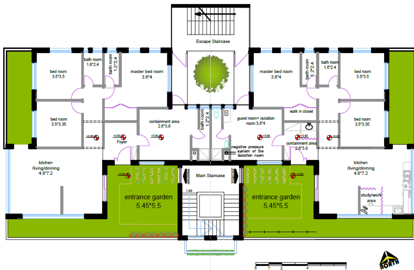
Figure 5: The proposed mirrored model is based on the common apartment plan. The figure provides a detailed architectural layout that integrates the entrance garden with internal corridors, designed to facilitate cross-ventilation and promote psychological well-being during confinement. These drawings provide the necessary spatial evidence for the dual vertical circulation system—comprising a main staircase and a dedicated 'Safe Path' escape staircase—which is a core requirement for health-resilience.
